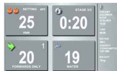
An easy-to-read status display shows the process temperature, the remaining cooking time, the mixer speed and the volume of water used.
