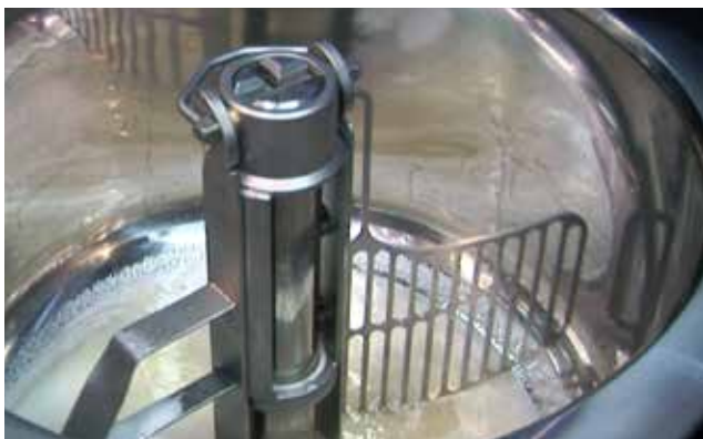
The mixer tool consists of three separate parts. The picture shows the whipping assembly.
