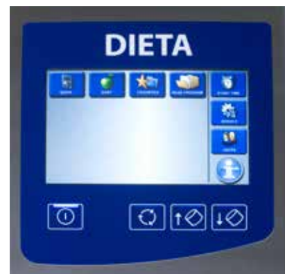
Start menu: Choose from four main directories – QUICK, EASY, FAVOURITES and READ PROGRAM.
